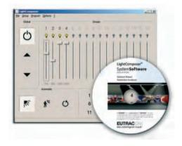
**The LightComposer software,** a special development for **EUTRAC** DALI, allows intuitive start-up and operation of the system including feedback informations. Options exist to dim and switch luminaries to control light scenes and create interactive actions or special automatic sequences.
